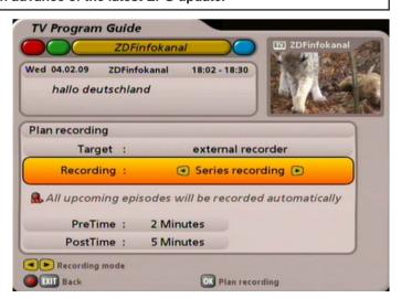
When all settings have been made, press the or button to save the recording settings. You can view the scheduled recordings in the recording schedule view of the EPG (see item "Recording schedule").
